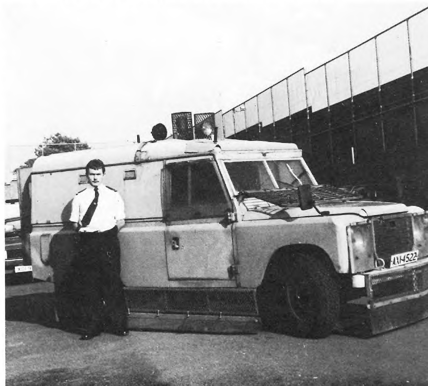
● Below: A long wheelbase LandRover fitted with an armoured body and special glass, and used for normal patrol work. The 'skirt' prevents explosive devices being rolled underneath the vehicle.
