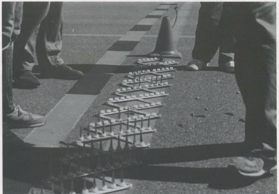
Researchers inspect the 'road fangs' after a vehicle has been driven across the device.
