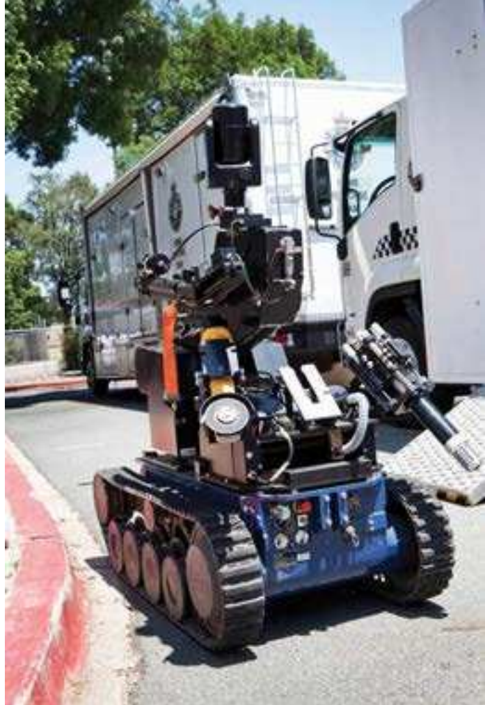
The tEODor bomb response robot is the largest of the AFP's six platforms.
