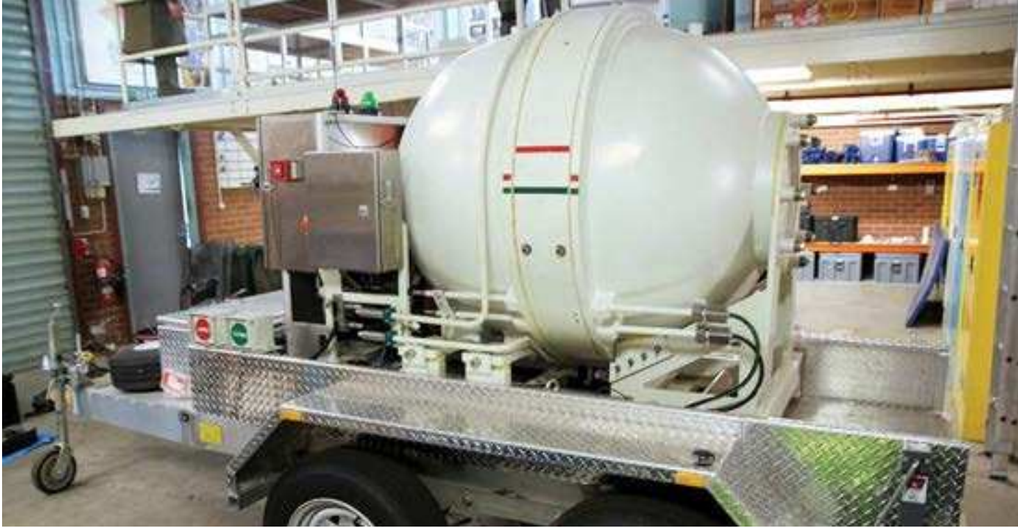
The trailer-mounted total containment chamber can safely confine a detonation of hazardous explosive materials.
