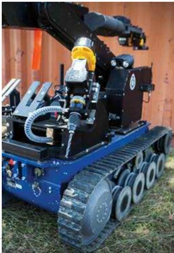
A tEODor bomb response robot changes tools by remote control.
