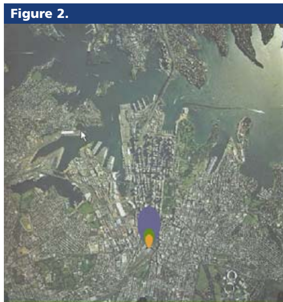
Figure 2: The dispersion of a radioactive plume resulting from a hypothetical detonation of a dirty bomb (40 GBq americium-241 source; 1kg TNT) over Sydney. The scenario was modelled using Hotspot™ software code. The defined regions represent the predicted 50-Year Committed Effective Dose Equivalent (CEDE) in Sieverts from the plume, received by an individual remaining at a specific location during the radioactive material release. The red represents a CEDE greater than 10 mSv, the green represents a CEDE of greater than 5 mSv, and the blue represents CEDE of greater than 1 mSv. Photograph © Department of Lands (2004).
