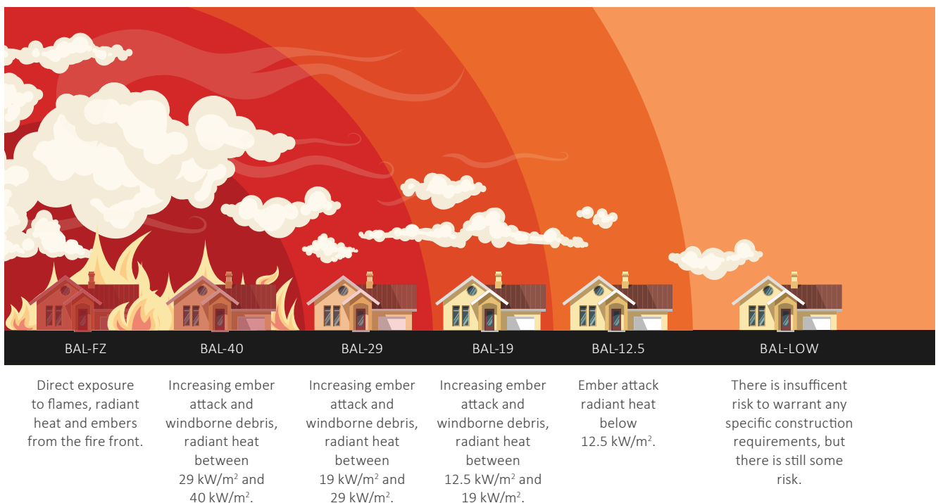
Figure 1: Bushfire Attack Level ratings indicate a building’s potential exposure to bushfires and the severity.
