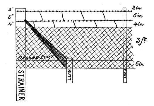
Strainers not less than about six inches in thickness at smaller end, one hundred and fifty yards apart, three feet in the ground, forty-nine inches out of ground.
